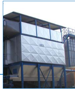
Extraction in a rotary drum furnace of an aluminum recycling plant Air volume: 90,000 Nm 3 /h — Temperature 170 °C
